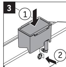
> Place tank on housing and fully insert hose in opening.
